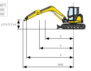
The lifting capacity is based on the ISO 10567 and it does not exceed more than the 75% of static tipping load or more than the 87% of the hydraulic lifting capacity of the machine.
