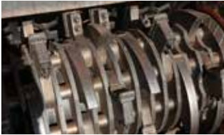
Hammermill System with (18) hammers, (18) rakers, and (18) inserts
