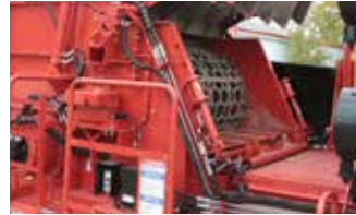
Extended Maintenance Platform
