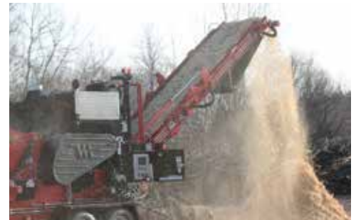
Optional folding conveyor with 14' 6" (4.42 m) load height
