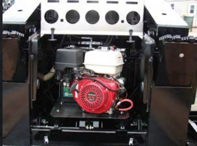
Pony Motor with Controls on Neck
