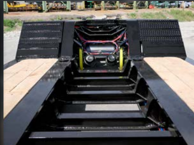
Boomwell in Main Deck (Dropped Crossmembers)
