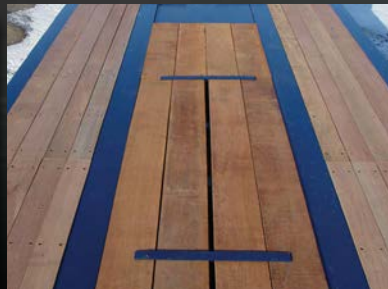
Outrigger Boards & Hold Down Kit
