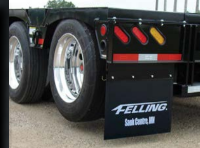
Strobe Light Kit & Lift Axle
