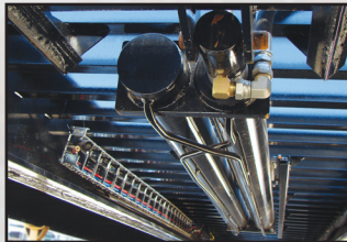
STD. 4.5" Dual Ram Slide Axle Cylinder - Retracted Slide Axle Cylinder in Transport Position
