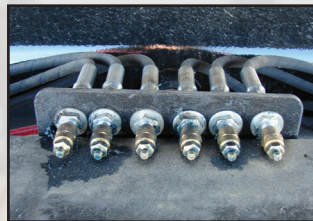
STD. Central Grease Zerk location - located at the rear of the trailer
