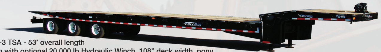
FT-80-3 TSA - 53' overall length shown with optional 20,000 lb Hydraulic Winch, 120" deck width, wireless remote for winch, 255R22.5 tires & white paint
