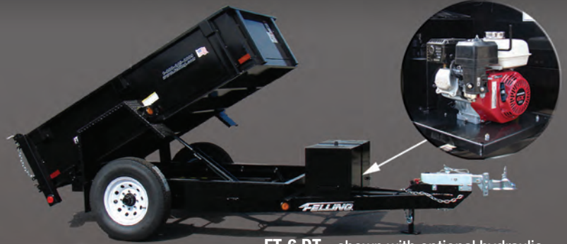
FT-6 DT - shown with optional hydraulic surge brakes & gas engine (in lieu of electric/hydraulic pump) 39504
