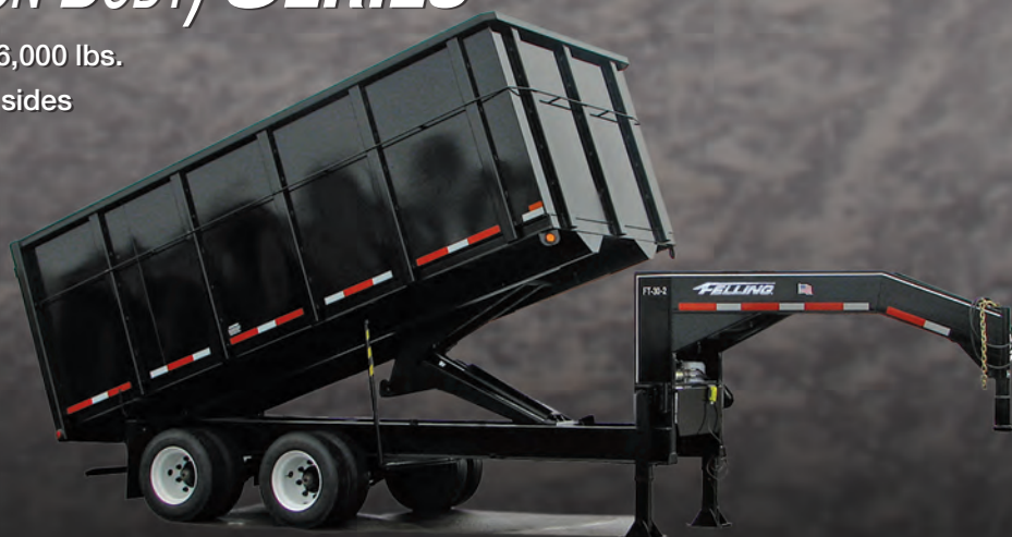
FT-30-2 DT DO Construction Body - shown with optional gooseneck coupler & tie rail around dump box 31833
