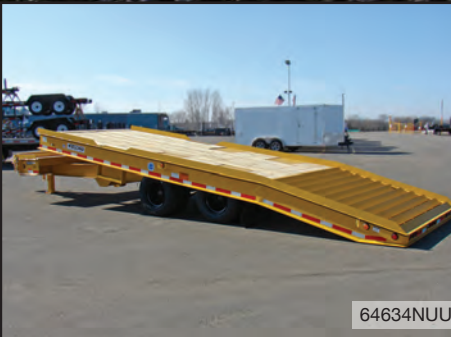
Custom Hyd. Tilt: 2' stationary deck, oak decking w/angle on last 72", custom beavertail, 4" x 3/8" lip up, yellow paint
