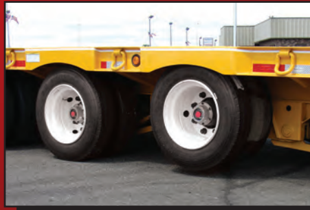
Air lift axle (requires air ride)
