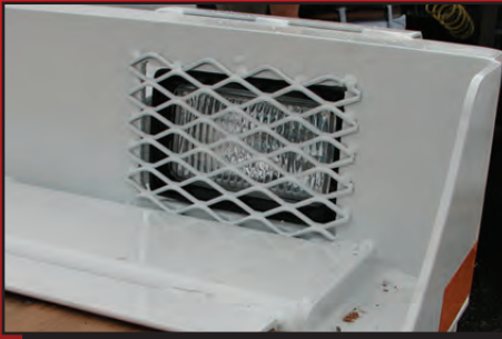
Loading lights in safety bulkhead
