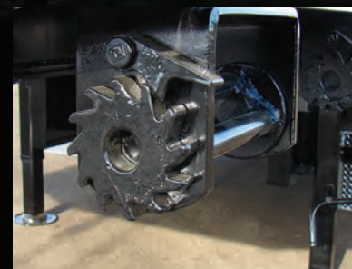
Weld on Winch
