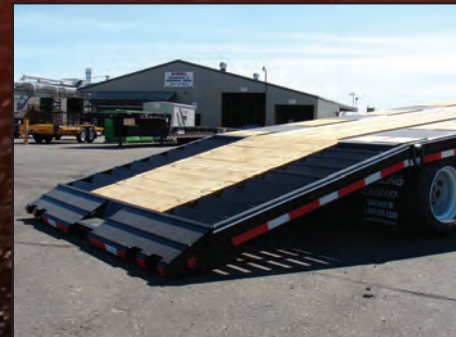
6' beavertail 5" x 3" self-cleaning angle on outer edges with oak center
