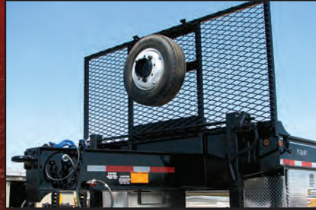
4' mesh headache rack w/spare tire
