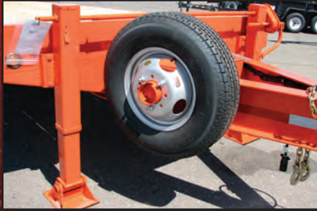
140K twin 2-speed jacks w/spare tire
