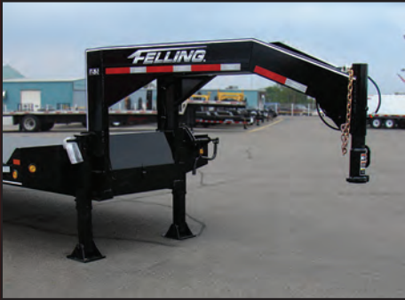
2 - 5/16" gooseneck coupler hitch
