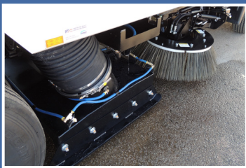
VACUUM AND BRUSH REMOVAL OF DEBRIS
