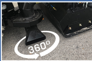
HIGH VELOCITY BLAST AIR TO PUSH MATERIAL OFF SURFACE
