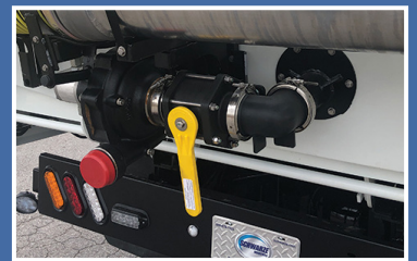
GLYCOL RECOVERY FOR PICKING UP DE-ICING FLUID
