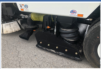
VACUUM AND BRUSH REMOVAL OF DEBRIS
