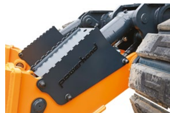
Well Protected Hydraulic Cylinders
