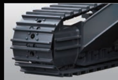
3 Heavy duty shoe (700 mm double bar grouser)
