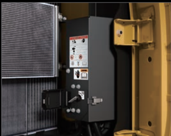
Battery Disconnect Switch with DEF Purge Notification Light
