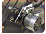
After resting the sweeper on the ground, remove the pins from motor and bearing mounts
