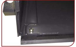
Additional steel reinforcement/welds between bolts and cutting edge and side plates
