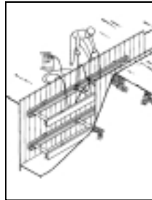
Disconnect lifting sling. Disconnect hose with release tool.
