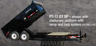
The Stationary Platform Option can be selected on any of Felling's Hydraulic Dump Model Lines.
