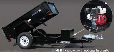
FT-6 DT - shown with optional hydraulic surge brakes & gas engine (in lieu of electric/hydraulic pump) 39504
