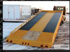
Custom Hyd. Tilt: 2' stationary deck, oak decking w/angle on last 72", custom beavertail, 4" x 3/8" lip up, yellow paint Custom Hyd. Tilt: front 3/4 tread plate, rear 1/2 self-cleaning angle w/oak center, 2" x 2" x 3/16" tube rail along deck, yellow paint
