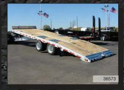
Custom Air Tilt: galvanized, sliding 4" belt winch & track for sliding belt winch, grouser bars over wheels
